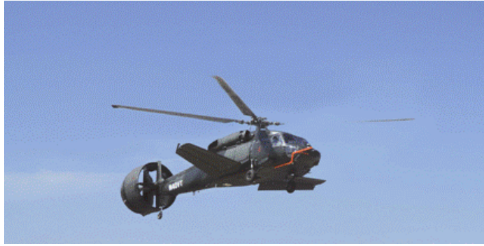
Piasecki's military-funded X-49A. Note the aircraft wing, five blade propeller and controllable ring-tail
