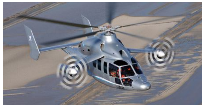
Eurocopter's X3 uses two propellers that provide forward thrust. Power for these propellers comes from the main engine.
