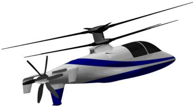
Sikorsky's X2 design is basically a helicopter with coaxial main rotors
